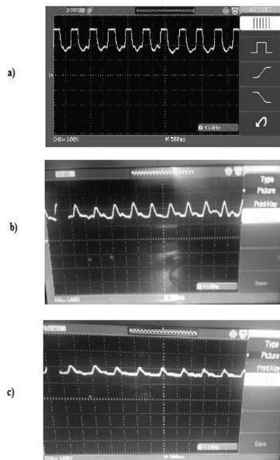
Figure 2. PPG output waveforms from a) index finger, b) palm and c) ear.
